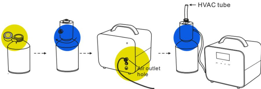
1. Wrap the neck of bottle with PTFE tape to seal it and screw the bottle to the atomizing head;
