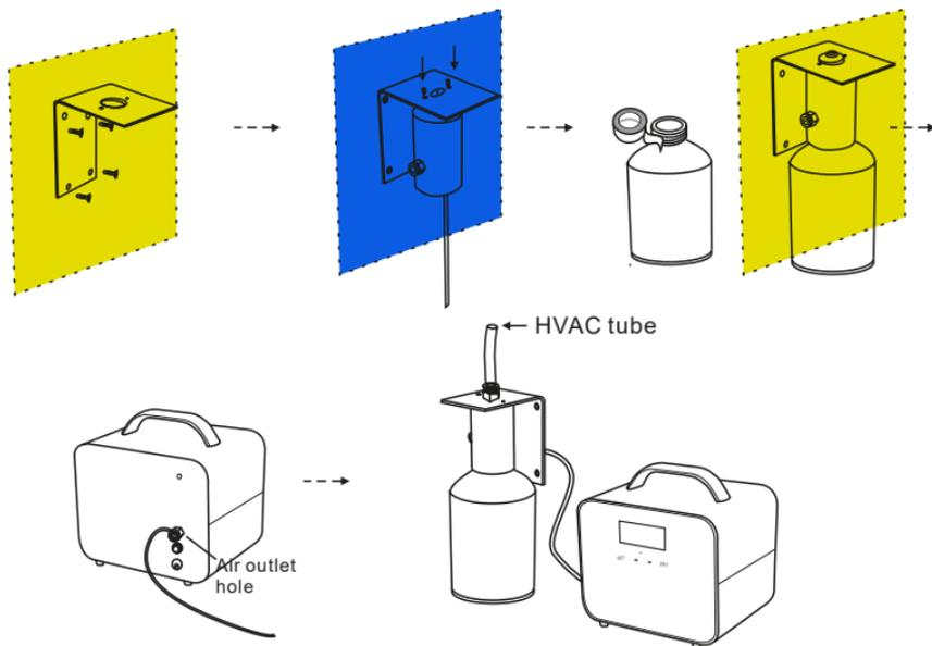
1. Use the screws to fasten the mounting bracket to the wall.
